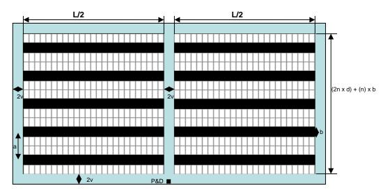
Figure 1 - Manual-Picking Order Picking System Layout
